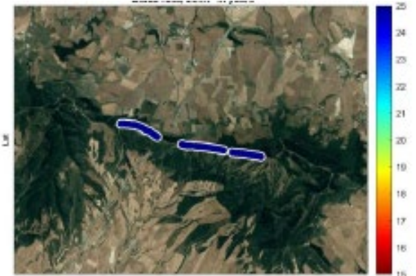
Wind farms P50 life estimation map for the component “Blade root, Joint” in years
