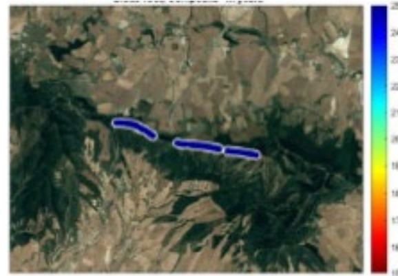
Wind farms P50 life estimation map for the component “Blade root, Composite” in years
